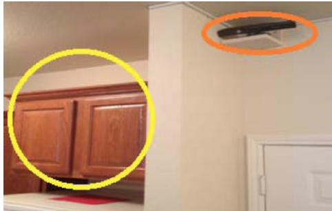
Fig. 13. The system setup at TigerPlace. The Kinect sensor is positioned over the front door of the apartment and the computer is placed inside the cabinet highlighted in yellow. (For interpretation of the references to colour in this figure legend, the reader is referred to the web version of this article.)
